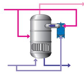
The plate evaporator installed as a booster to an existing effect
