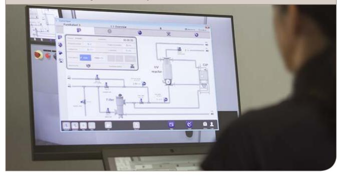
Alfa Laval PureBallast 3 Computer-Based Training (CBT) is an online/offline training tool that serves as a complement to face-to-face crew training. It combines self-study in ballast water management with a 3D simulation of the Alfa Laval PureBallast 3 ballast water treatment system (see reverse), as well as a self-assessment.
